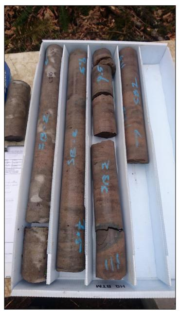
Typical Basalt Coring Observed on the Site (SB-2, 5-15'BGS).
