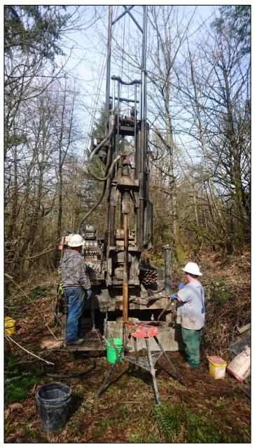
**Conducting Soil Boring Exploration (SB-2).**
