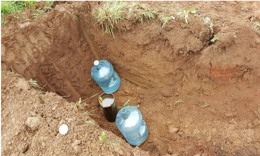
Infiltration Testing in Test Pit TP-1
