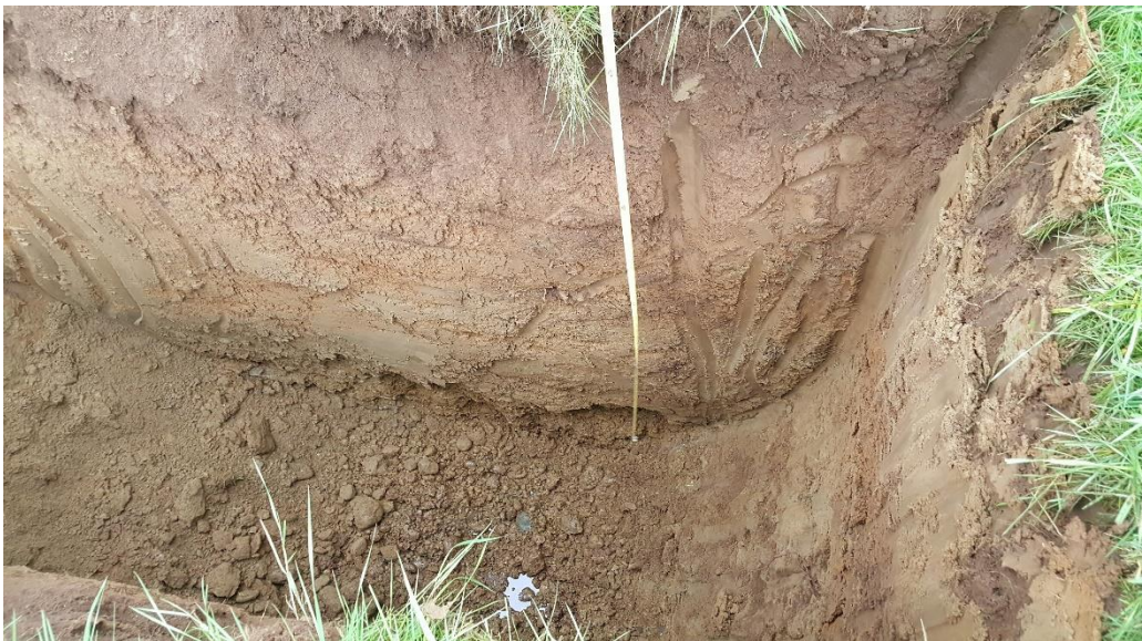
Test Pit Exploration TP-2, Competent Gravels Observed at Groundwater Elevation
