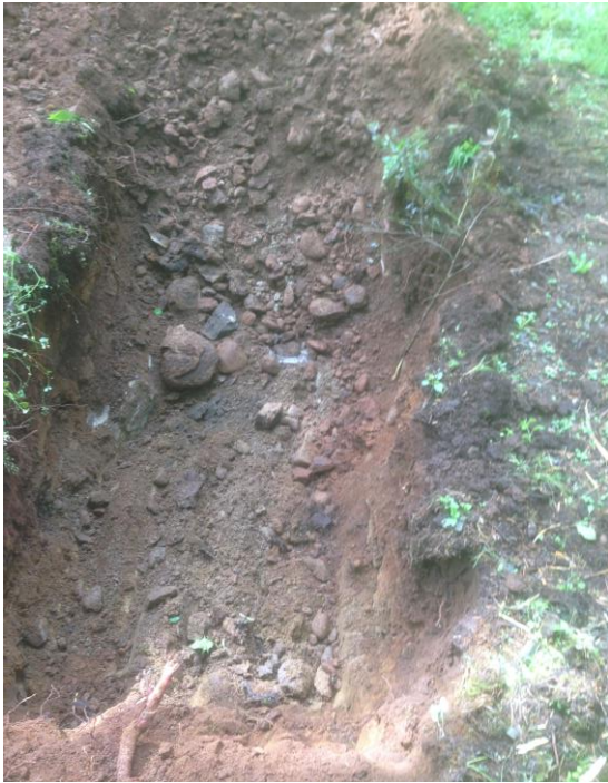
Shallow conglomerate bedrock in Test Pit TP-1
