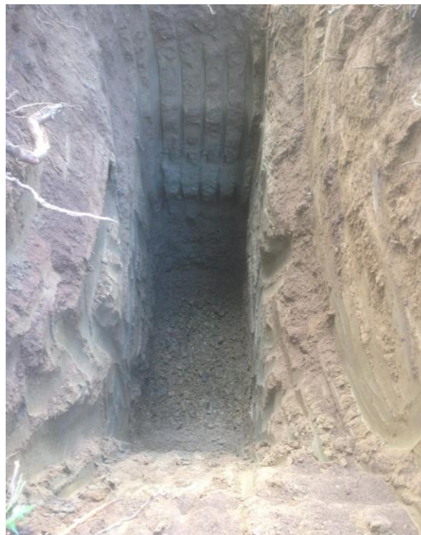
Deeper conglomerate bedrock encountered in Test Pit TP-8
