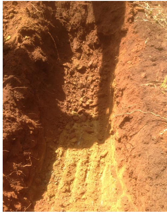
Shallow hyaoclastic sandstone bedrock in Test Pit TP-3
