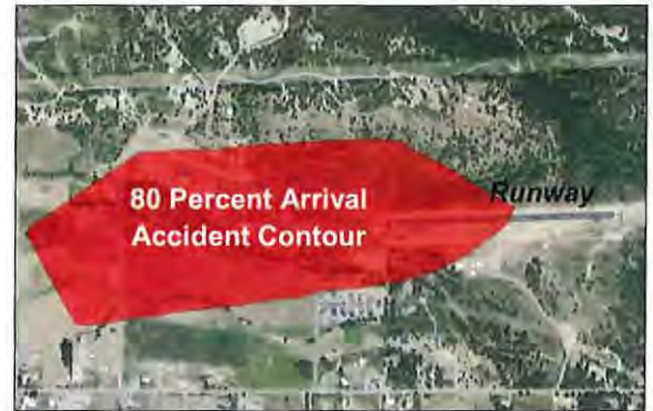
Historic accident distribution contours were georeferenced and overlaid on this community airport's runway end using GIS. Data Source California Airport Land Use Planning Handbook, 2002
