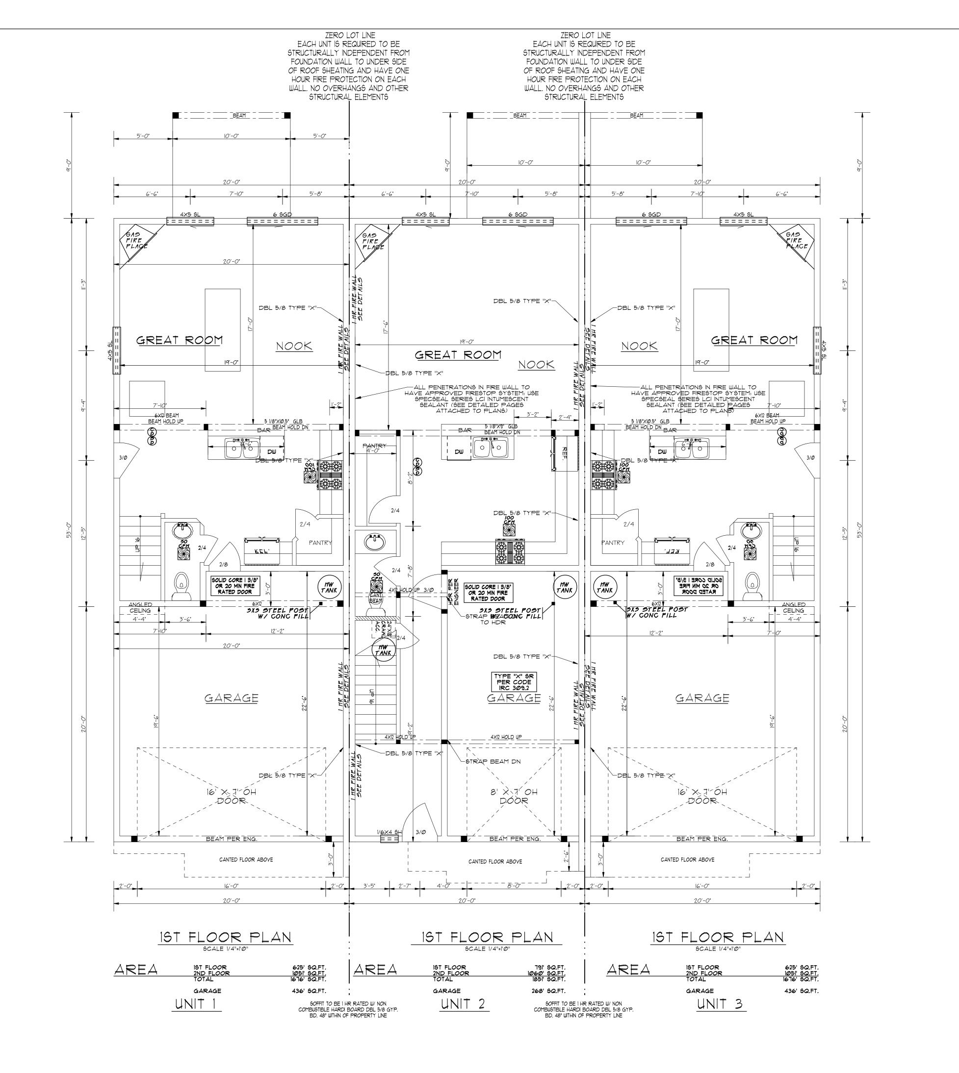
Note: Blackened Area = Posts or Studs = 6x6 Posts or (3)2x6= 4x6 Posts or (3)2x4=  $4\times4$  Posts or  $(2)2\times4$ To be determined by framer unless specified on the plan. MIN. LOADS FLOOR: IN PSF ECKS: in PSF LIVE 40lbs. DEAD 20lbs. LIVE 251bs. DEAD 171bs. .IVE 40lbs. DEAD 1016s. 6x8 hdr min. 7'-9" ceilings unless noted on plan 4x10 hdr min. 8'-0" ceilings unless noted on plan 4x10 hdr min. 9'-0" ceilings unless noted on plan
